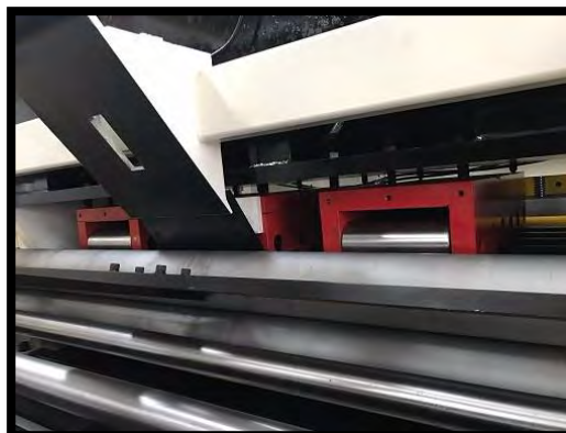
GCr15 steel rolls, HRC 60
